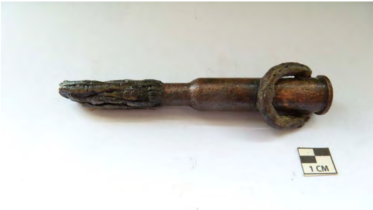
Tool used for field maintenance of the Lewis M20 machine gun (Dutch). A very rare find.
